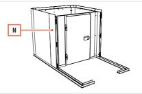
Position the ceiling panel  $(\mathbf{0})$  by wedging it between the wall panel profiles.
